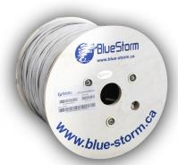
BlueStorm 23AWG Cat6A 500MHz UTP Solid Bare Copper Ethernet Cable is high-speed cabling specifically designed for use in 10GBase-T (10Gbps) indoor network environments. Constructed using 23AWG solid pure bare copper conductors with a PVC jacket and a cross separator, it exceeds TIA/EIA 568-C.2 standards and it is safe for use in the Riser spaces of commercial class buildings. This cable is RoHS compliant.
